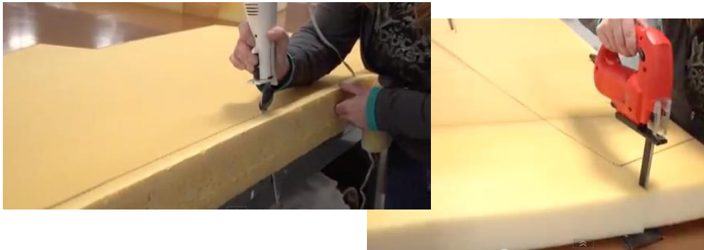
Cutting a Foam Wedge with an Electric Knife and Using a
