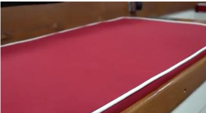
Using Piping to Finish the Edges
