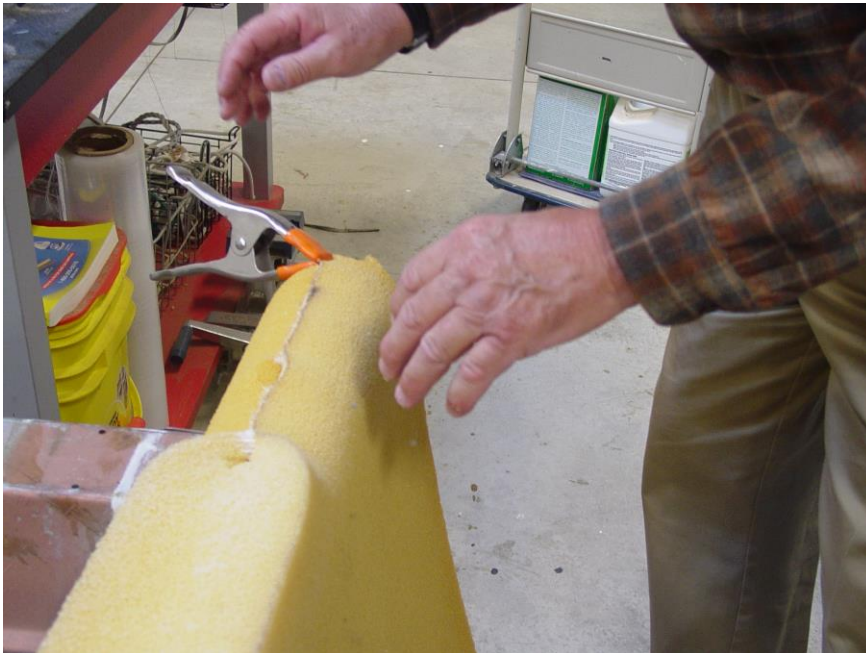
Creating a Rounded Edge in Four Inch Open Cell
