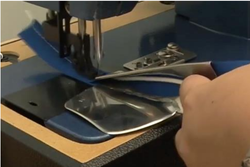
Using a 2 Inch Swing Binder to Make Piping
