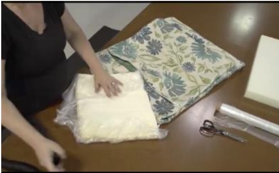
The Hose Has Been Removed — The Foam Is Much Smaller than the Pocket
