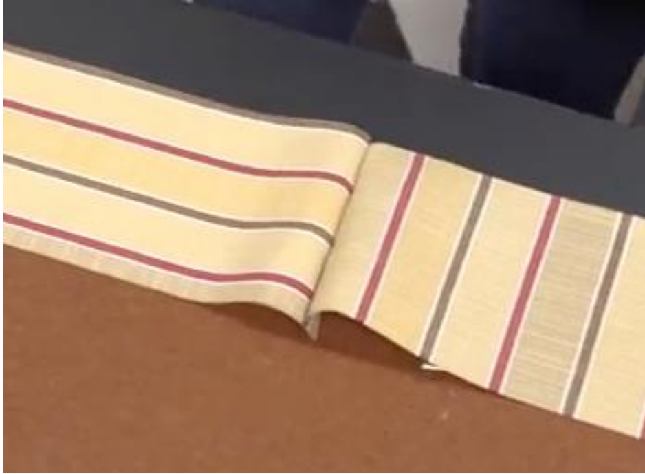
Two Boxing Segments Attached with a Semi-Flat Felled
