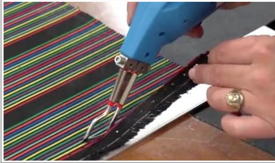
Trimming Excess Width Beyond the Nominal
